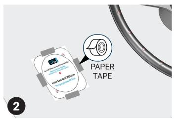
2. Place the "FILOS Drilling Pattern" in the desired position, preferably a clean and easy-to-access area, close to the vessel's steering wheel.
