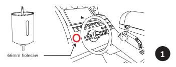
Use 66mm holesaw to create a hole in the desired position.
