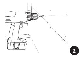
Open the 4 holes (Figure 2), and mount the AIR Unit by tightening firmly the screws.
