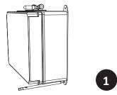
Place the unit in the desired position at the inner of the boat and make the marks that will be used to drill the holes for the mounting scews.
